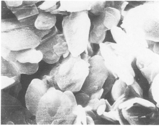
Fig. 10. SEM of boron nitride-coated surface.
